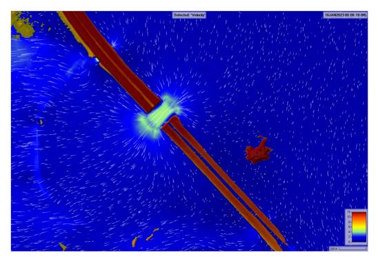
Figure 3.1.2.2E Bridge #4 & Culvert #4 100-Year Velocity
