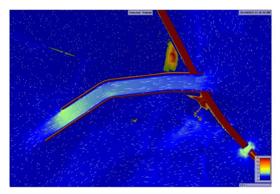
Figure 4.3D. 500-yr Velocities and Flow Patterns for Proposed Floodplain Bridge and Channel
