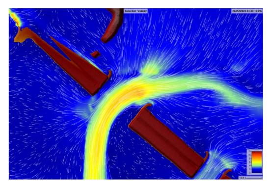
Figure 4.2E. Bridge #3 Velocities and Flow Patterns (500-Yr) with Guide Banks
