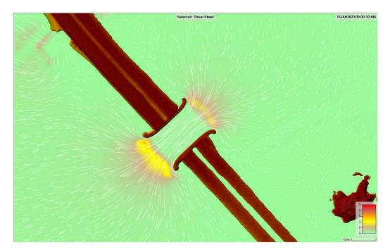
Figure 4.21. Bridge #4 Shear Stress (100-Yr), Guide Banks
