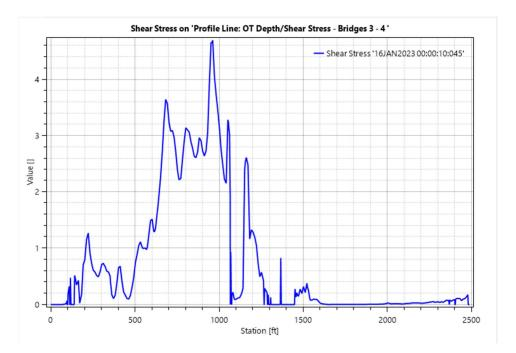
Figure 3.1.2.1G. 100-Year Overtopping Shear Stress, Shoulder of EB Lanes
