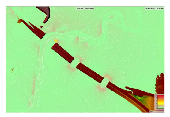
Figure 3.1.2.2D Bridges #1-3 500-Year Shear Stress
