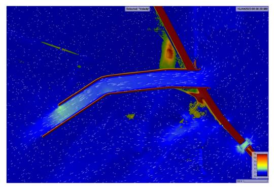
Figure 4.3C. 100-yr Velocities and Flow Patterns for Proposed Floodplain Bridge and Channel
