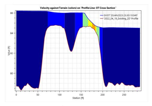
Figure 3.1.2.1K. 500-Year Water Surface & Terrain Example Across Overtopping Location
