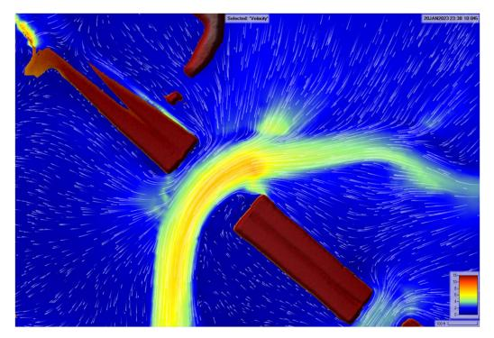
Figure 4.2D. Bridge #3 Velocities and Flow Patterns (500-Yr), Existing Conditions
