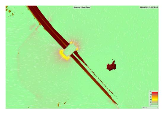
Figure 3.1.2.2H Bridge #4 & Culvert #4 500-Year Shear Stress
