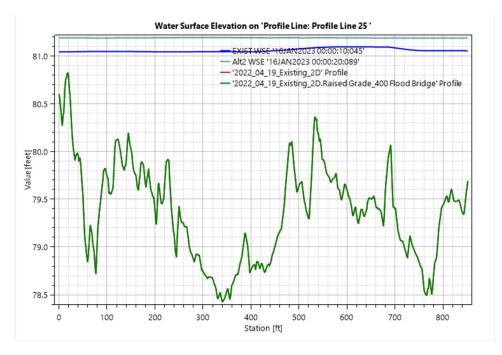
Figure 4.3M. 100-Yr Water Surface Elevation Comparison at 20296 NC-130
