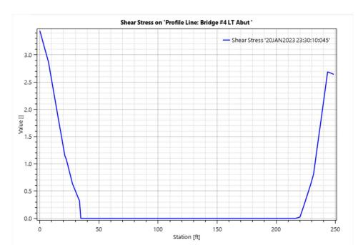
Figure 4.20. Bridge #4 Left Abutment Shear Stress (500-Yr), Guide Banks
