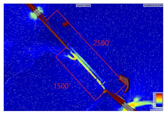
Figure 3.1.2.1I. 500-Year Overtopping & Velocities (Bridge #3 to Bridge #4)
