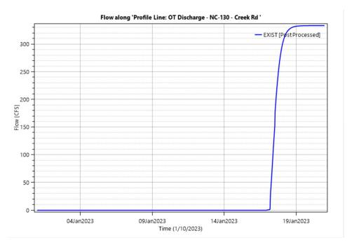
Figure 3.1.2.1T. Overtopping Flow Across Shoulder of EB Lanes (NC-130 to Creek Rd.)
