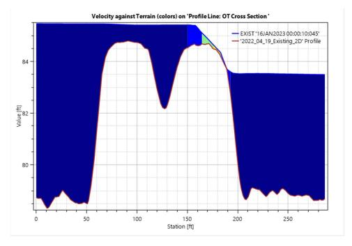
Figure 3.1.2.1F. Example Roadway Cross Section with 100-year Water Surface & Velocity
