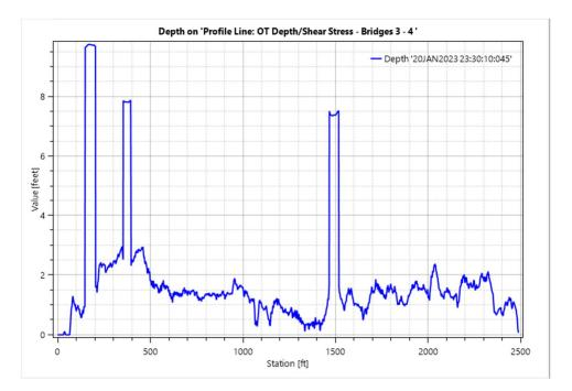
Figure 3.1.2.1J. 500-Year Overtopping Depth, Shoulder of EB Lanes (Bridge #3 to Bridge #4)
