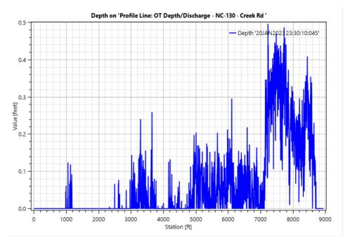
Figure 3.1.2.1P. 500-Year Overtopping Depth, EB Lanes (NC-130 to Creek Rd.)
