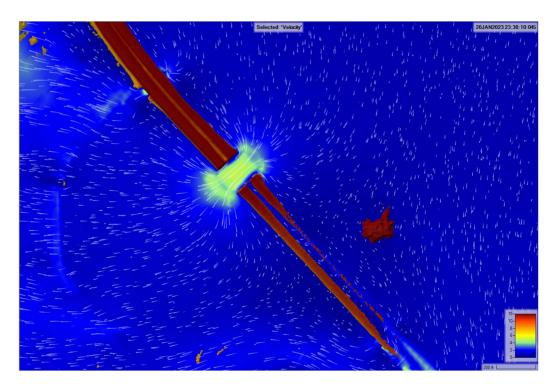
Figure 3.1.2.2F Bridge #4 & Culvert #4 500-Year Velocity
