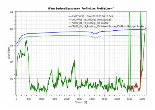
Figure 4.3F. 100-Yr Water Surface Elevation Comparison Along Upstream Embankment
