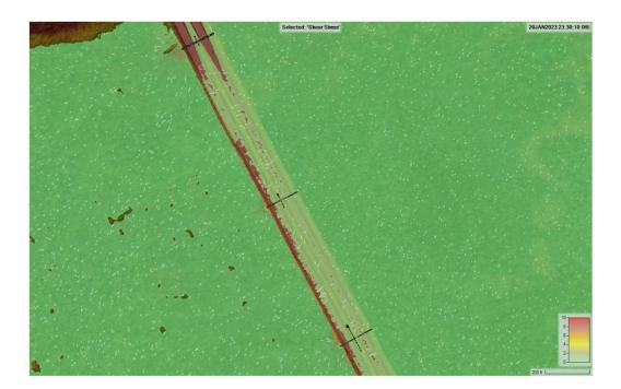
Figure 3.1.2.1R. 500-Year Shear Stress (Pipe #5 - Pipe #7)
