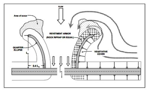
Figure 4.2A. Typical Guide Bank Example (HEC 23)
