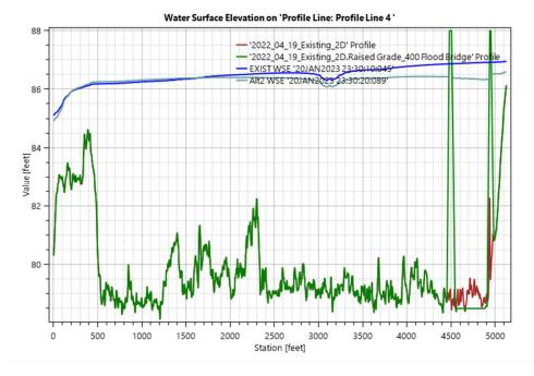
Figure 4.3G. 500-Yr Water Surface Elevation Comparison Along Upstream Embankment
