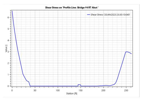
Figure 4.2Q. Bridge #4 Right Abutment Shear Stress (500-Yr), Guide Banks
