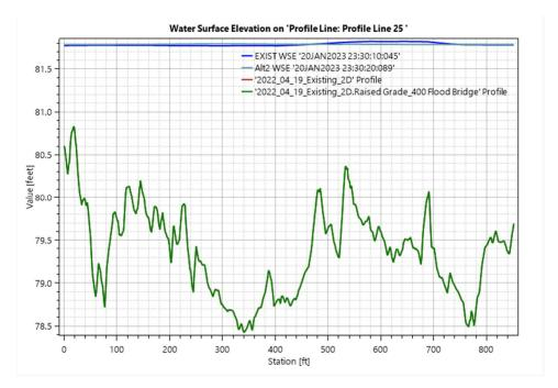
Figure 4.3N. 500-Yr Water Surface Elevation Comparison at 20296 NC-130
