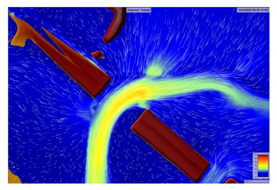
Figure 4.2B. Bridge #3 Velocities and Flow Patterns (100-Yr), Existing Conditions
