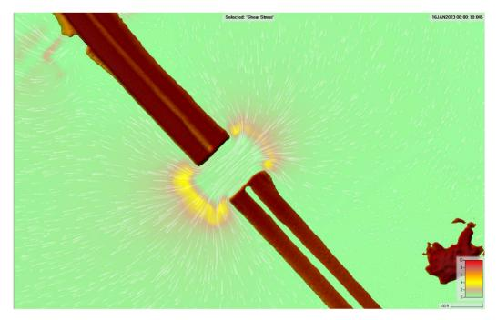
Figure 4.2H. Bridge #4 Shear Stress (100-Yr), Existing Conditions
