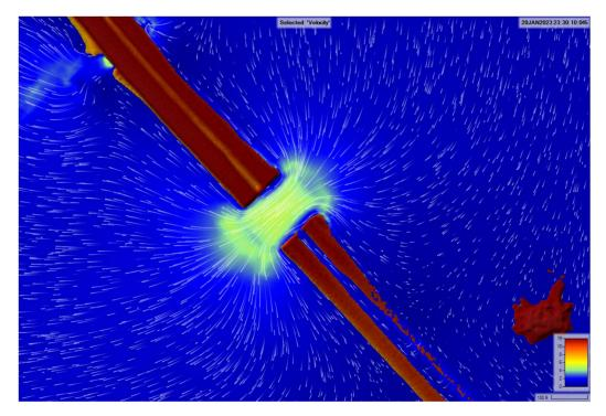
Figure 4.2J. Bridge #4 Velocities and Flow Patterns (500-Yr), Existing Conditions
