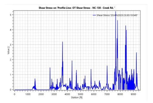
Figure 3.1.2.1Q. 500-Year Overtopping Shear Stress, Shoulder of EB Lanes (NC-130 to Creek Rd.)
