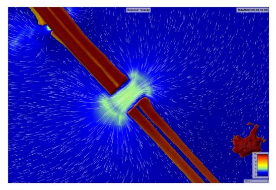
Figure 4.2F. Bridge #4 Velocities and Flow Patterns (100-Yr), Existing Conditions
