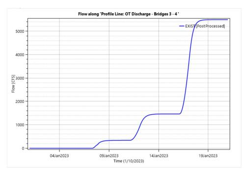
Figure 3.1.2.1S. Overtopping Flow Across EB Lanes (Bridge #3 to Bridge #4)
