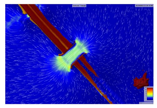
Figure 4.2K. Bridge #4 Velocities and Flow Patterns (500-Yr), Guide Banks
