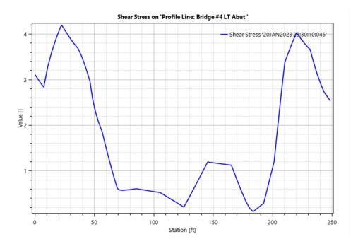
Figure 4.2N. Bridge #4 Left Abutment Shear Stress (500-Yr), Existing Conditions
