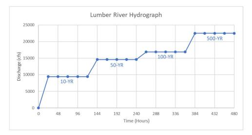
Figure 3.1.1A. Stepped Flow Hydrograph Upstream Boundary Condition on Lumber River
