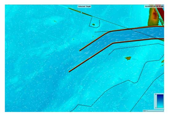
Figure 4.3K. 100-Yr Depth and Flow Patterns at 20296 NC-130 with Flood Channel
