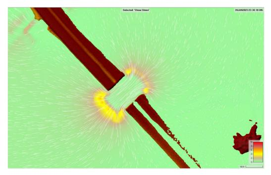
Figure 4.2L. Bridge #4 Shear Stress (500-Yr), Existing Conditions
