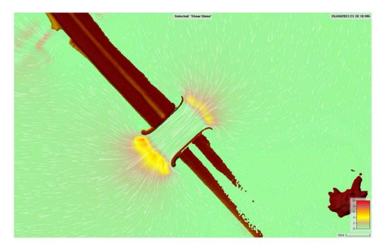
Figure 4.2M. Bridge #4 Shear Stress (500-Yr), Guide Banks
