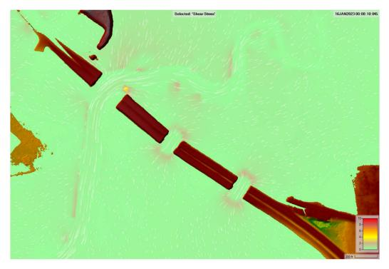
Figure 3.1.2.2C Bridges #1-3 100-Year Shear Stress
