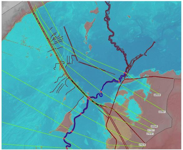
Figure 3.1.3 FEMA 1D Cross Sections
