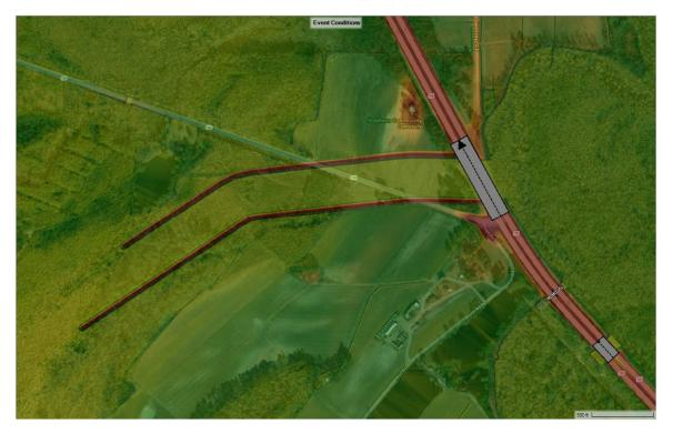
Figure 4.3A. Proposed Floodplain Bridge and Channel in RAS Mapper
