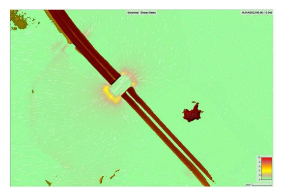
Figure 3.1.2.2G Bridge #4 & Culvert #4 100-Year Shear Stress
