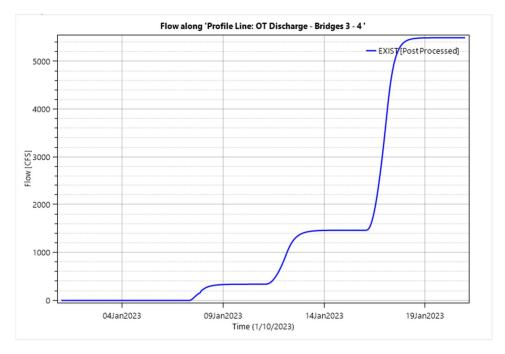
Figure 4.3H. Overtopping Flow Between Bridges #3 & #4 (Existing)
